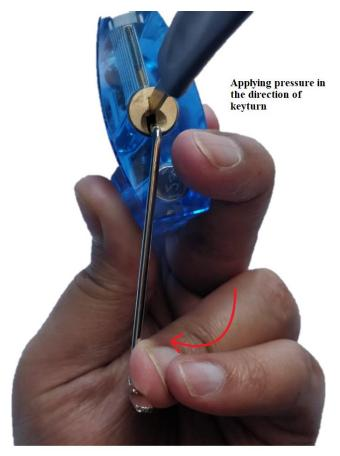
**4. Balance the pins using hook:** Once the position is attained, we try to balance the pins and then when they are in place, the lock opens, **and we have physical access.** The entire process takes only 5-10 minutes at the hands of an expert
